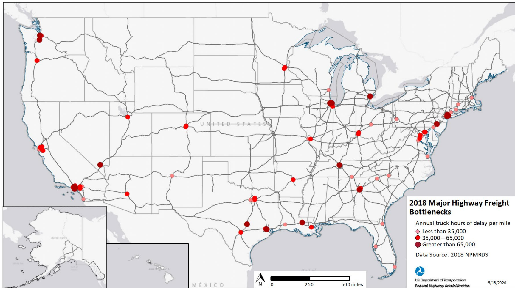
Map-1. Major Freight Highway Bottlenecks Based Upon Truck Hours of Delay per Mile, 2018 NPMRDS
