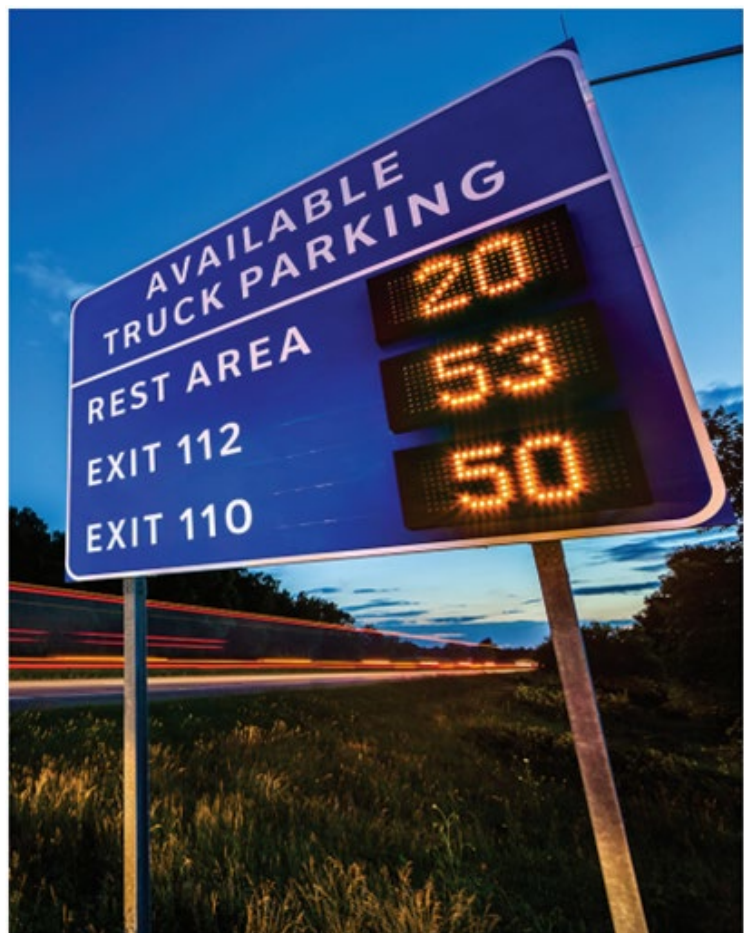
Figure 7: A dynamic messaging sign used to display the number of available parking spaces at rest areas in Michigan. Source: Michigan DOT. (Untitled). (No date).
