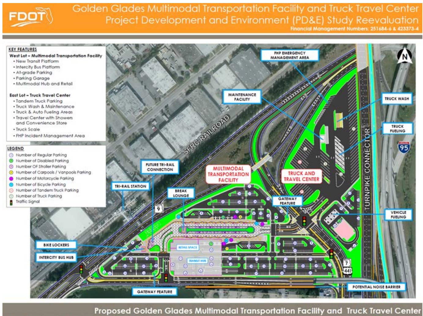
Figure 8: Proposed design of Golden Glades Multimodal Transportation Facility and Truck Travel Center. Source: FDOT.
