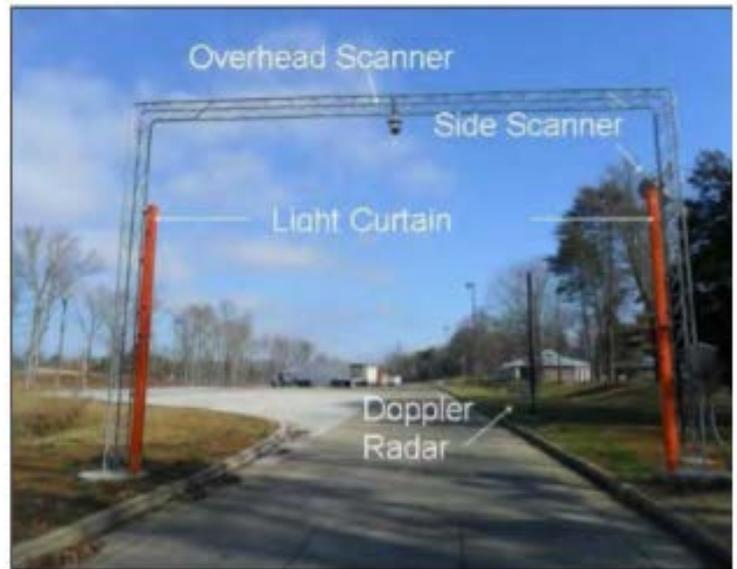
Figure 5: SmartPark detector configuration. Source: <https://www.tn.gov/content/dam/tn/tdot/documents/RES2016-08.pdf>.
