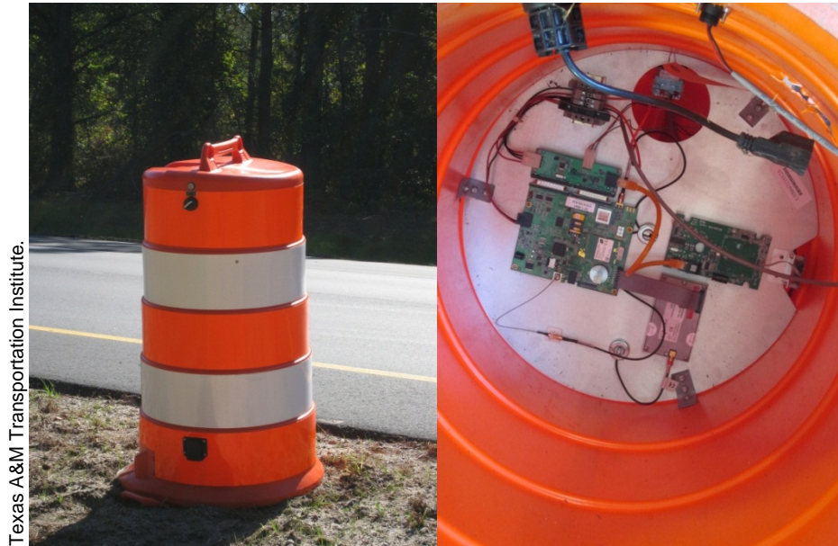
Figure 5. Photo. iCone® Portable Traffic Monitoring Devices.
