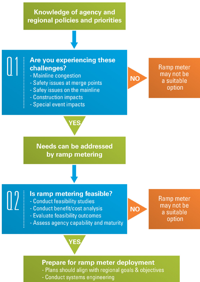
Figure 9: Ramp metering deployment decision process flow
