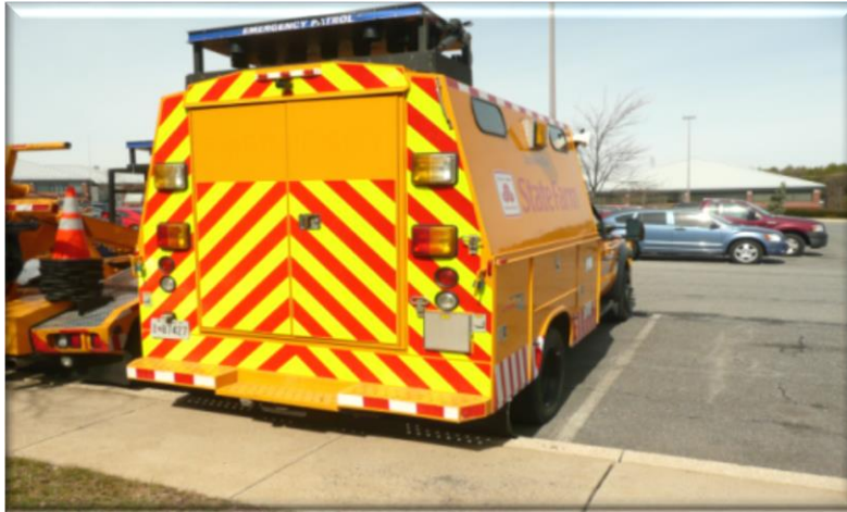
Figure 8. Photo. Example of Rear Conspicuity Striping. Source: Maryland State Highway Administration
