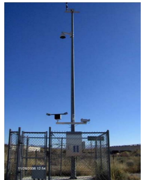
Figure 1. Visibility sensor in Arizona Department of Transportation Dual Use Safety Technology Warning System. (Source: Arizona Department of Transportation)
