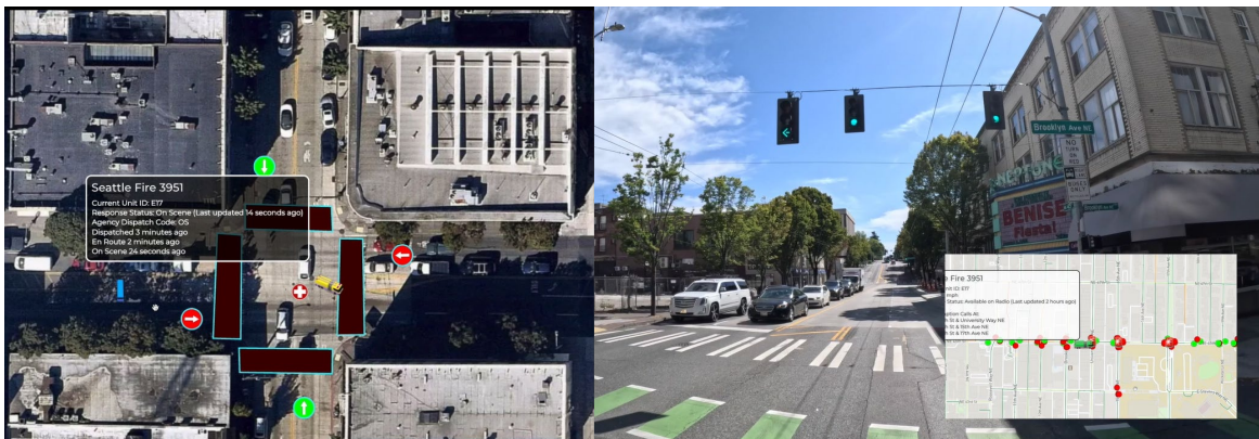
Figure 1: Seattle Fire Department vehicle receiving real-time cloud-based signal priority along a MICMA corridor
