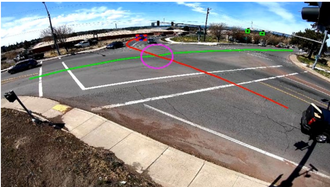
FIGURE 8.5: STREET SIMPLIFIED CAMERA IDENTIFYING A THROUGH-THROUGH NEAR-MISS EVENT AT NW ARIZONA & NW COLORADO
