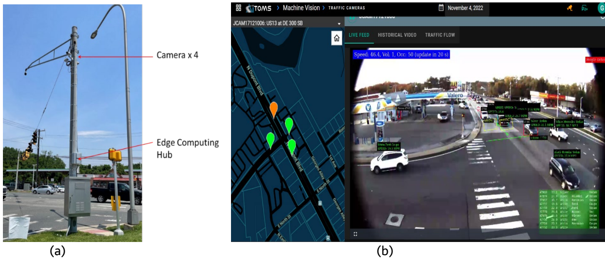
Figure 5. (a) BlueHalo’s Edge Computing multi-channel machine vision cameras installed at US-13 @ DE-300 in Smyrna, DE; (b) the web portal for the machine vision cameras for vehicle count, classification, and speed and occupancy estimation
