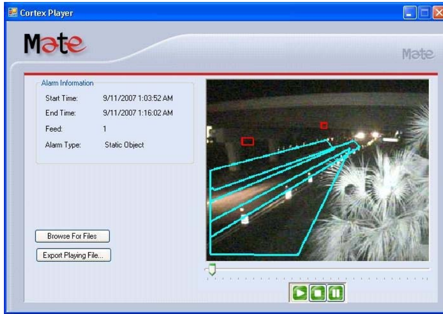
Figure 137. Example of a Bridge Security System False Alarm at Night
