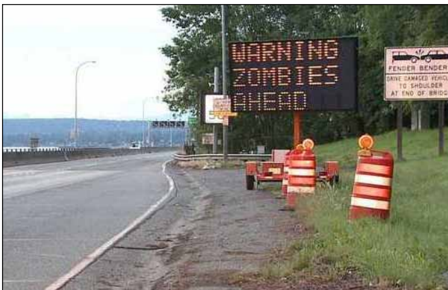
Figure 16. PCMS in several states have been illegally accessed and had messages changed.
