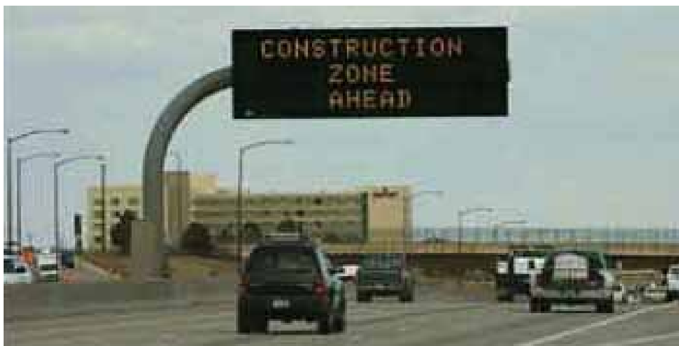
Figure 7. Existing ITS resources can be used to help manage the work zone and reduce costs.
