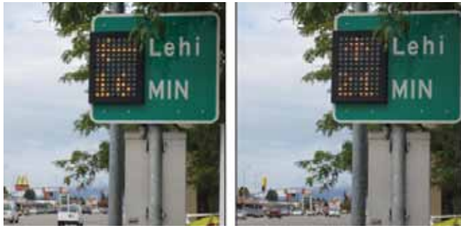
Figure 3. Sequencing comparative travel time sign at a decision point for two different routes to the town of Lehi that was used for a project in Utah.
