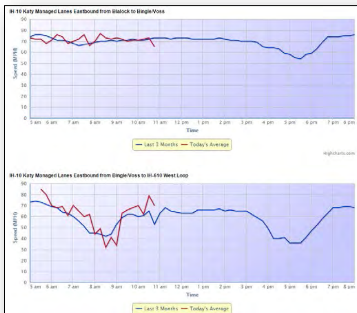
Figure 31. Illustration. Example of speed performance monitoring at Houston TranStar. (83)
