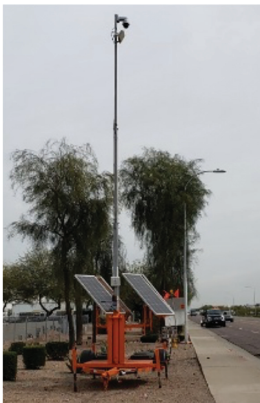
Figure 4. Smart Work Zone equipment with CCTV camera and Roadside Unit (Source: Maricopa County Department of Transportation)
