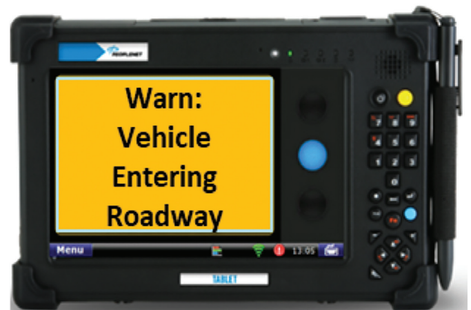
Figure 5. In-vehicle messages provided about the work zone (Source: Maricopa County Department of Transportation)
