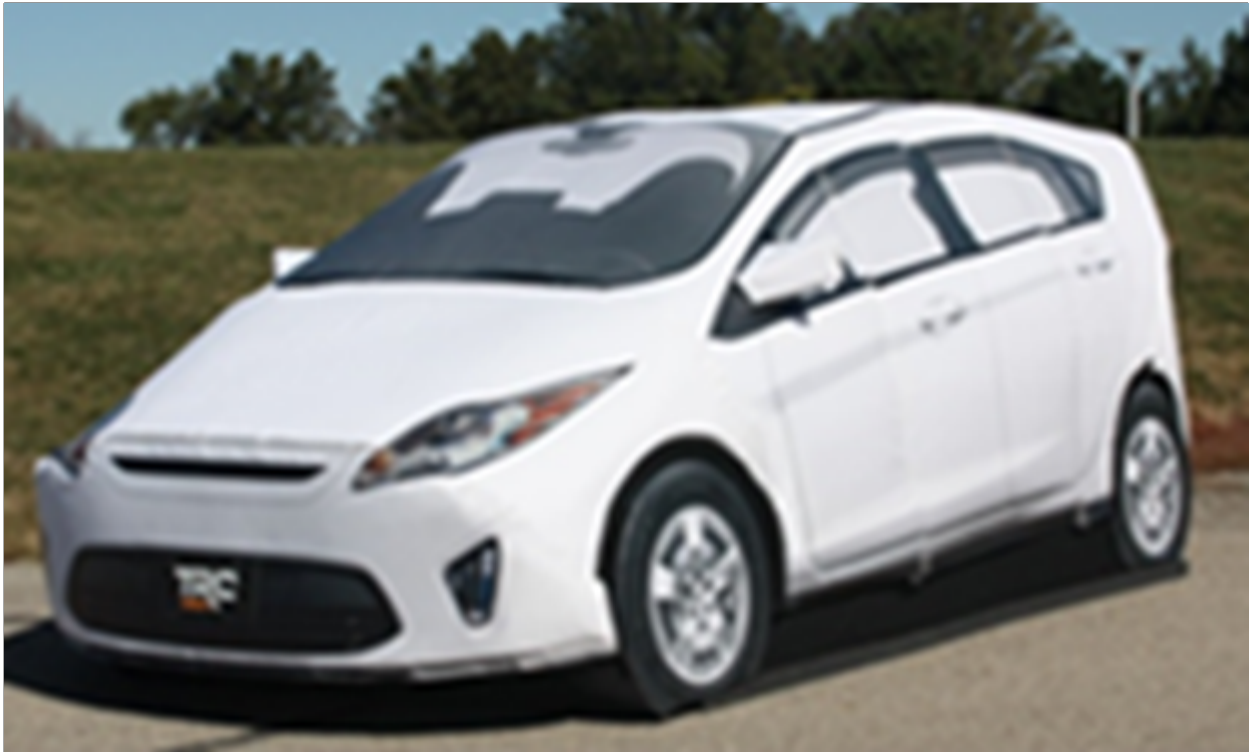
Figure 24. Photo. Soft Car used for Stopped Car Detection scenario in the Winter FT#2.
