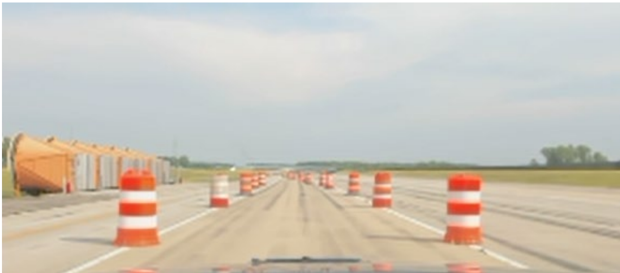
Figure 12. Photo. Test vehicle point of view depicting work zone barrels and crosswind generators. Barrels were placed such that the crosswind generators were at the start of the taper.
