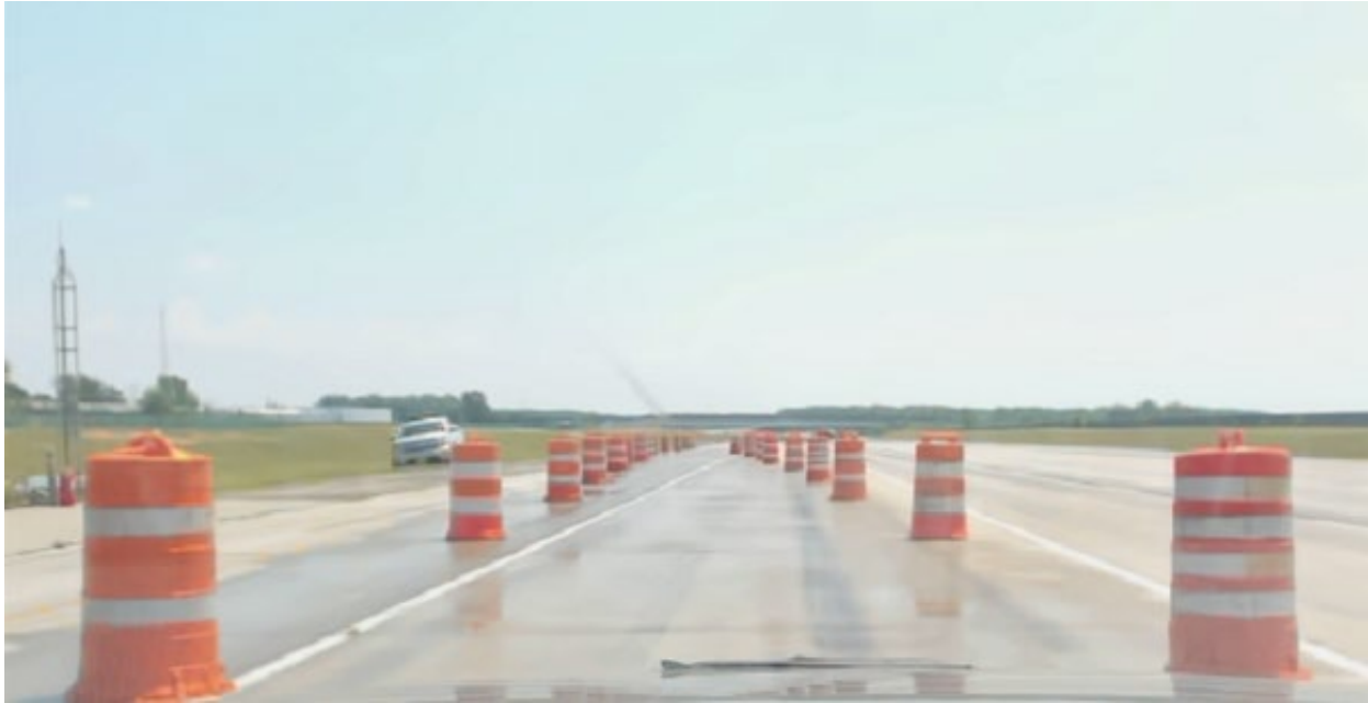
Figure 9. Photo. Test vehicle point of view depicting Work Zone Lane Change with Barrels scenario with wet pavement conditions and sun glare during daytime testing.
