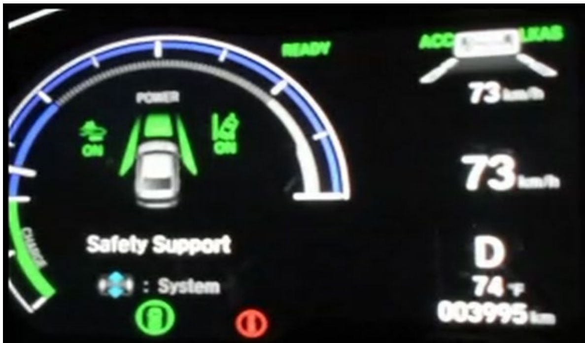
Figure 1. Photo. Summer FT#1 Vehicle A's HMI displaying support systems that were engaged during the testing.
