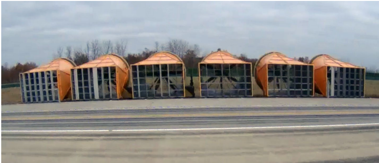
Figure 7. Photo. Wind Generators used for Work Zone Lane Change with Barrels scenario in Summer FT#1.
