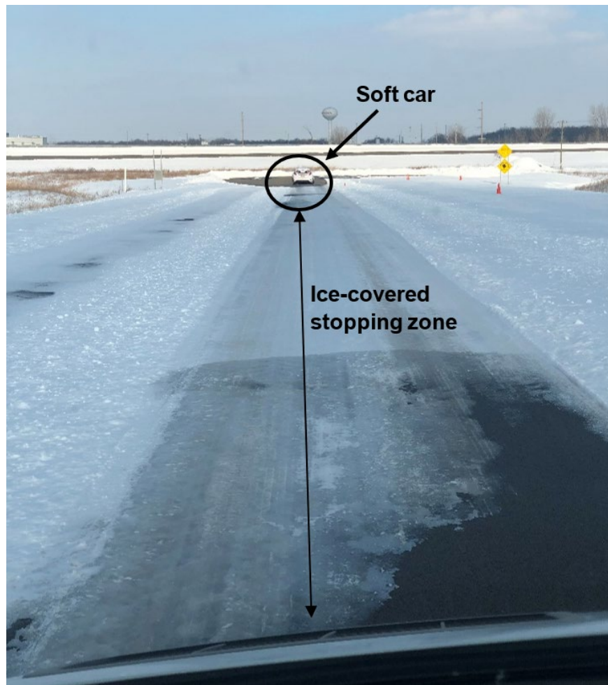
Figure 36. Photo. Ice-covered stopping zone on the travel lane of Vehicle A and stopped soft car.
